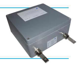
Solid state polarization cells or AC grounding devices are used to mitigate pipeline AC voltages resulting from induction from overhead power lines sharing the same corridor.
